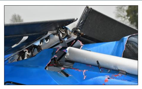
Photo No. 3: Fractured central keel tube
