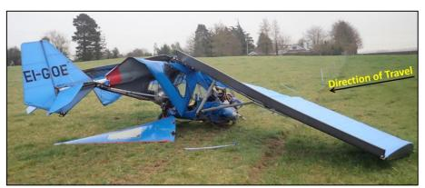
Photo No. 2: Final resting position of EI-GOE and damage sustained
